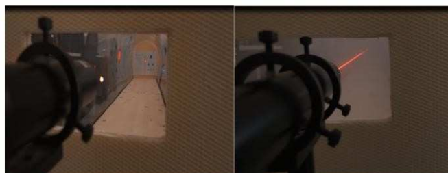
Fig. 9 – Measurements through 3m of fog a). low fog b). dense fog
