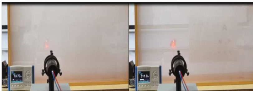
Fig. 10 – Measurements through 30 cm of fog a). dense fog b). low fog
